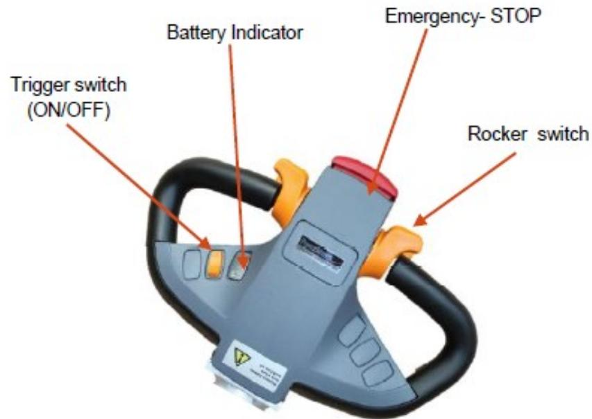
Tiller Head with Rocker switch and Emergency Button
