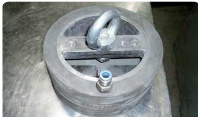
Pipe grip with external expansion
